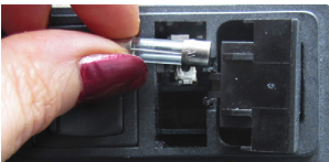
Fig. 17—Open the fuse housing and rotate it right to remove the fuse.
