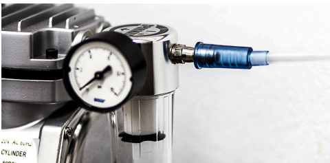
Fig. 4—Use the silicone suction connector to join hard tubing to a vacuum pump.
